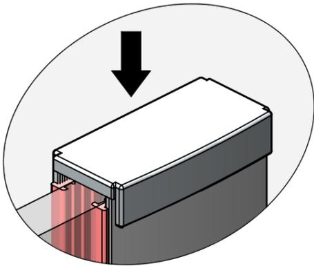
METTRE EN PLACE LE(S) CAPUCHON(S) DU PROFILÉ MURAL (PIÈCE 4). UNE PETITE QUANTITÉ DE SILICONE PEUT ÊTRE APPLIQUÉE SUR LA FACE INFÉRIEURE DU CAPUCHON POUR LE MAINTENIR EN PLACE SI NÉCESSAIRE.
